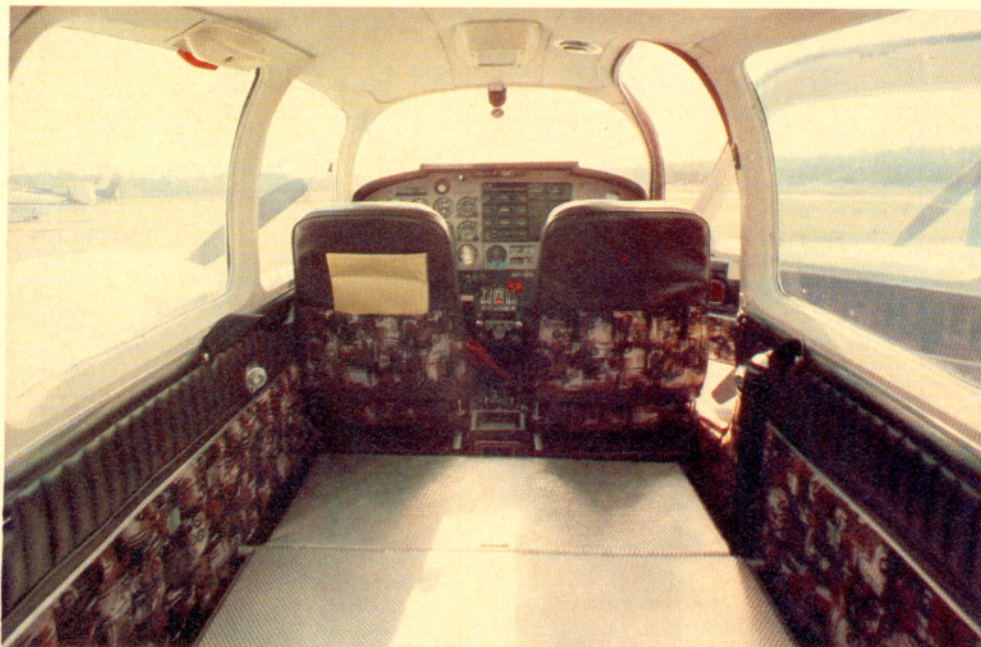
The Cougar's rear seat cushions are removable so seat backs can fold flat to extend the baggage compartment. Fuel selectors between the front seats are clearly marked, and have associated fuel pump switches close at hand.
