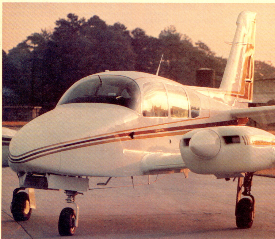
Twin 160-hp engines make for economy, although they produce cruise speeds up to 160 knots.
