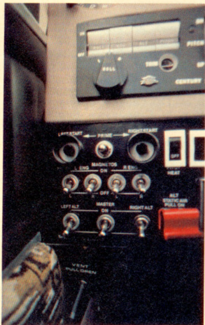
Primer, magneto, master and alternator switches, all similar, are in a tight array at lower left panel. The rest of the interior is both attractive and utilitarian.
