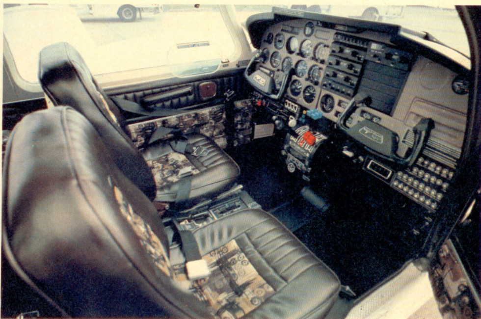
Primer, magneto, master and alternator switches, all similar, are in a tight array at lower left panel. The rest of the interior is both attractive and utilitarian.
