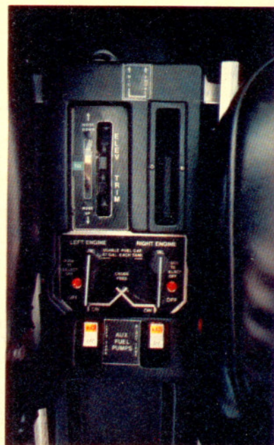
The Cougar's rear seat cushions are removable so seat backs can fold flat to extend the baggage compartment. Fuel selectors between the front seats are clearly marked, and have associated fuel pump switches close at hand.
